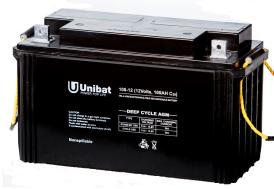
UNIBAT Deep Cycle AGM differs from conventional VRLA batteries, as it contains more lead, heavier plates and other special materials that enable to deliver more power and capacity over many charging cycles. The use of a special plate curing process for 10 days and extra superior pasting to the grids, ensuring long service life and fast recovery from deep discharge.
